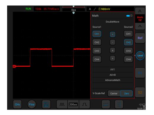
Figure 9-1 MATH Channel Waveform
