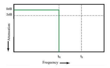
Figure 11-2 Theoretical Brick-Wall Frequency Response
