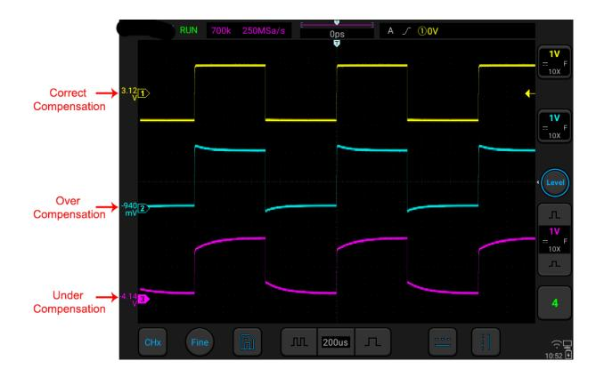
Figure 2-14 Probe Compensation
