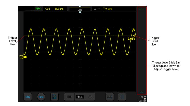
Figure 6-8 Trigger Level
