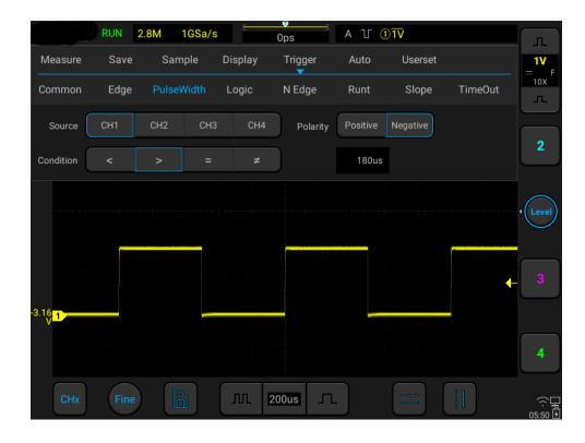
Figure 6-15 Negative Polarity Pulse Level Flip
