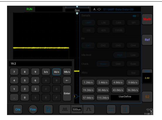
Figure 12-5 Baud Rate Default Setting
