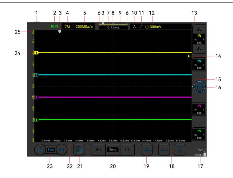
Figure 2-6 Oscilloscope Interface Display
