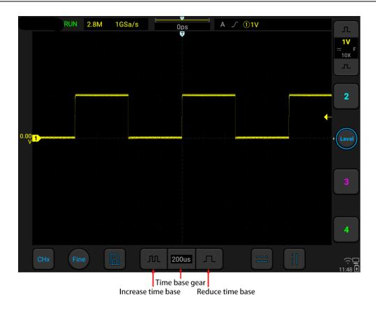
Figure 4-3 Adjust the Horizontal Time Base
