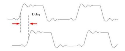
Figure 7-5 Delay Measurement Schematics
