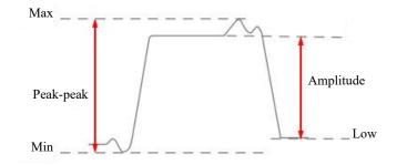
Figure 7-7 Voltage Measurement
