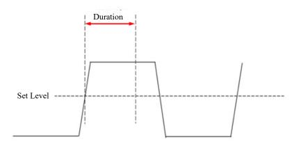
Figure 6-28 Timeout Trigger Schematics
