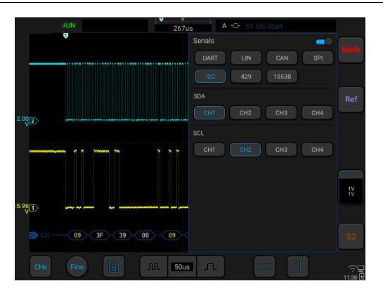
Figure 12-22 I2C Bus Configuration Menu
