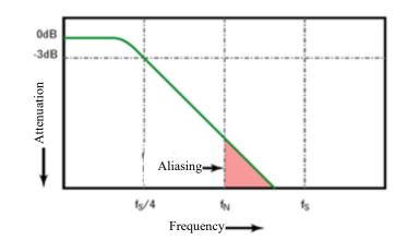
Figure 11-3 Sampling Rate and Oscilloscope Bandwidth
