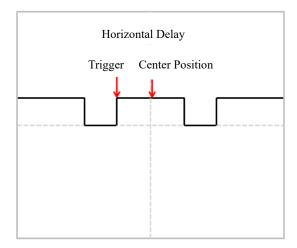
Figure 6-7 Horizontal Delay
