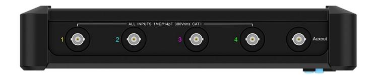
Figure 2-4 Top Panel of Tablet Oscilloscope
