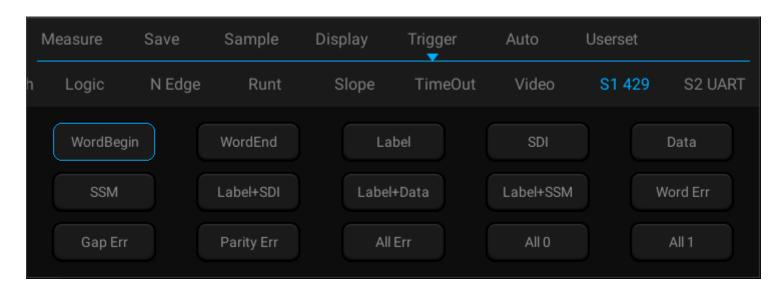
Figure 12-27 ARINC429 Trigger Mode Configuration Menu
