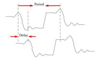
Figure 7-6 Phase Measurement Schematics
