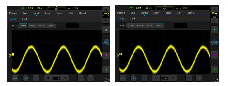
Figure 11-5 Sine Wave with Burr
