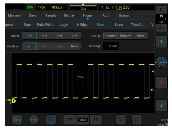
Figure 6-25 Runt Trigger Setting Menu
