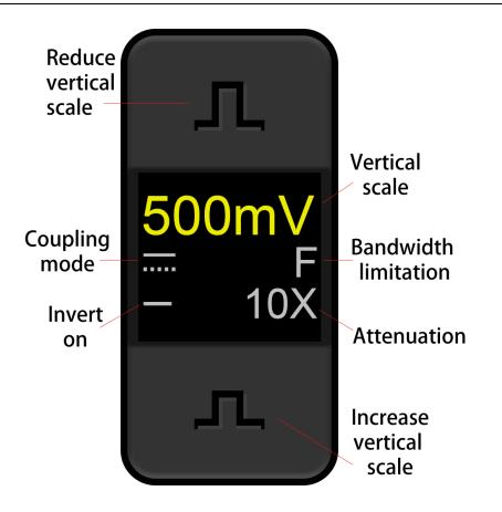
Figure 5-3 Channel Display Interface
