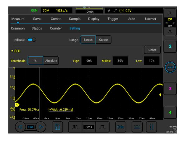
Figure 7-13 Set Middle Thresholds as 80%
