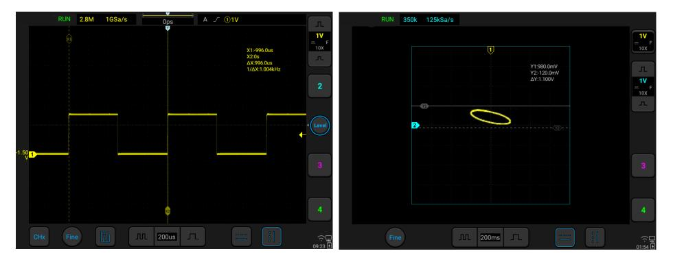
Figure 7-18 Cursor Measurement Pulse Width
