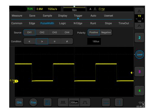
Figure 6-14 Pulse Width Trigger Setting Menu
