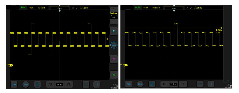
Figure 6-3 Abnormal Signal in Periodic Signals
