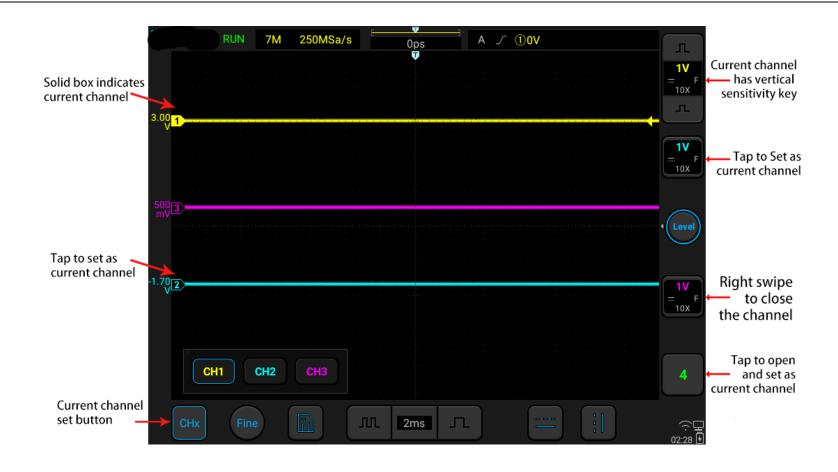
Figure 5-4 Channel Open, Close and Switching
