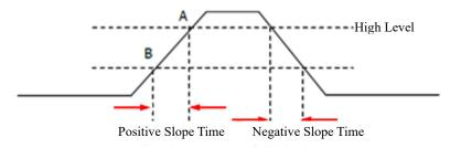
Figure 6-26 Positive/Negative Slope Time
