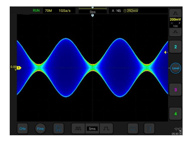
Figure 10-5 Color Temperature Open Mode
