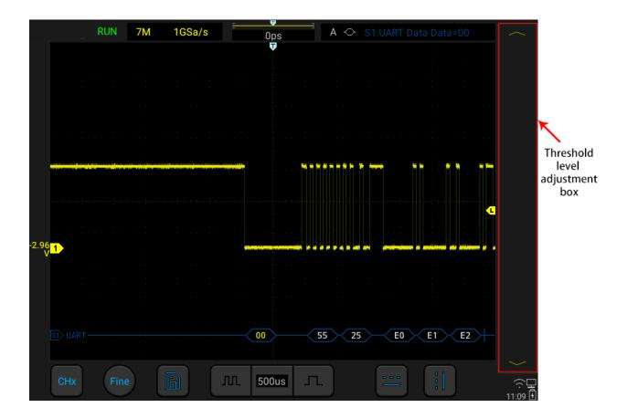
Figure 12-7 UART Decode Level Adjustment
