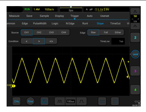
Figure 6-27 Slope Trigger Setting Menu
