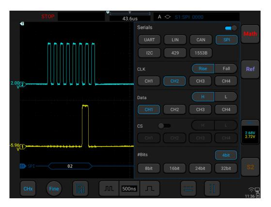
Figure 12-18 SPI Bus Configuration Menu
