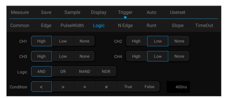
Figure 6-21 Logic Trigger Setting Menu
