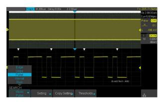
The GPS-2000XE can search events specified by the user in a frame. It can also navigate by time (delay position) and historical frames.
