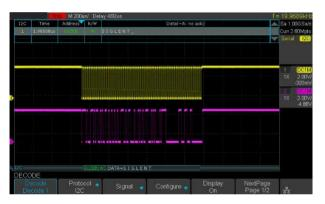
GPS-2000XE displays the decoding through the events list. Bus protocol information can be quickly and intuitively displayed in a tabular format.
