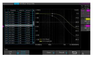
GPS-2000XE can control the USB AWG module or an independent GPS LTD SDG instrument, scan a circuits amplitude and phase frequency response, and display the data as a Bode Plot. It can also show the result lists, and export the data to a USB disk.
