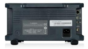
GPS-2000X -E supports USB Host, USB Device (USB -TMC), LAN, Pass/Fail and Trigger Out.
