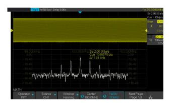
The new math co-processor enables FFT analysis of incoming signals using up to 1 million samples per waveform. This provides high frequency resolution with a fast refresh rate. The FFT function also supports a variety of window functions so that it can adapt to different spectrum measurement needs.
