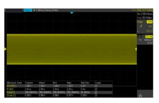
GPS-2000XE can apply automatic measurements on all sampled data points up to 28 Mpts. This ensures the accuracy of measurements while the math co-processor decreases measurement time and increases ease-of-use.
