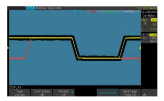
The GPS-2000XE utilizes a hardware-based Pass/Fail function, performing up to 40,000 Pass / Fail decisions each second. Easily generate user defined test templates provide trace mask comparison making it suitable for long-term signal monitoring or automated production line testing.
