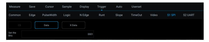
Figure 12-19 SPI Trigger Mode Configuration Menu
