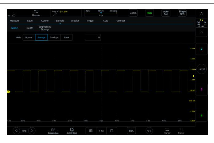
Figure 11-7 Waveform after choosing the average sampling mode, with average number 16
