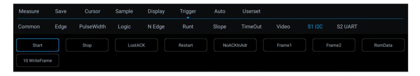
Figure 12-23 I<sup>2</sup>C Trigger Mode Configuration Menu
