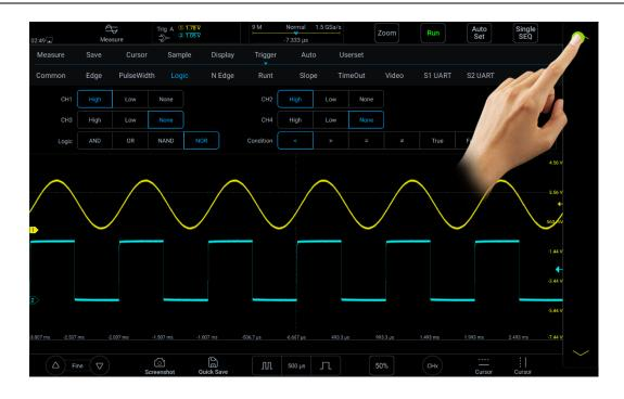
Figure 6-22 Trigger Level Adjustment
