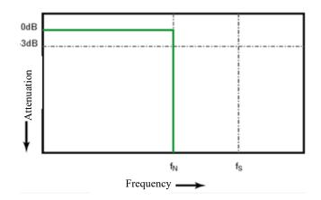
Figure 11-2 Theoretical Brick-Wall Frequency Response
