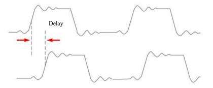
Figure 7-5 Delay Measurement Schematics
