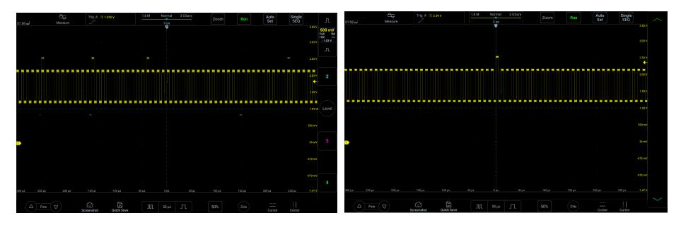
Figure 6-3 Abnormal Signal in Periodic Signals
