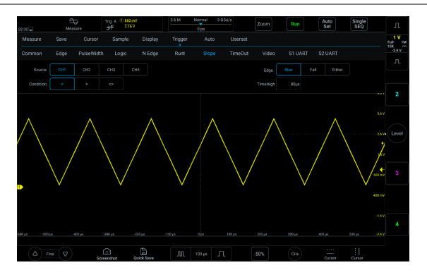
Figure 6-27 Slope Trigger Setting Menu
