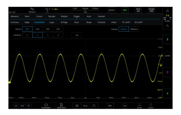
Figure 6-14 Pulse Width Trigger Setting Menu
