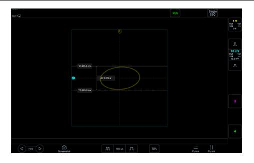
Figure 4-9 Phase Difference Measurement and Using the Cursor
