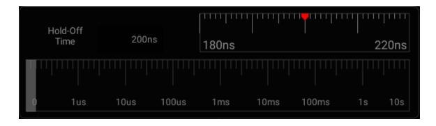
Figure 6-11 Trigger Hold-Off Time Set Interface
