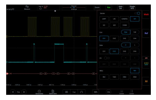
Figure 12-18 SPI Bus Configuration Menu
