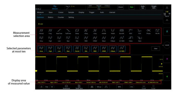
Figure 7-1 Automatic Measurement Menu
