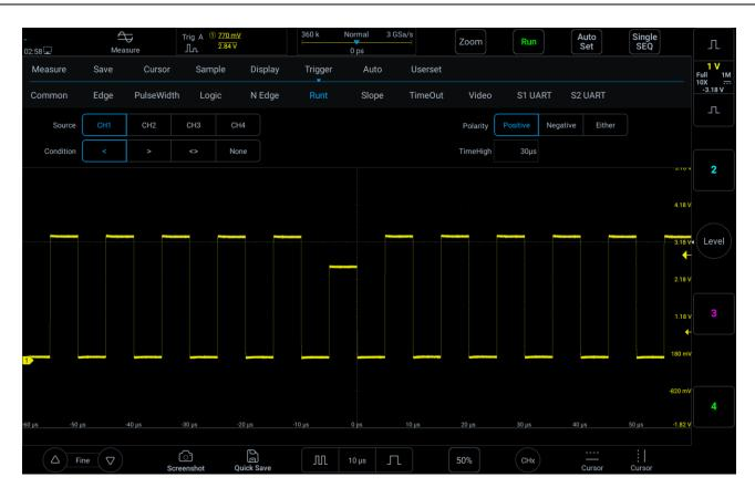
Figure 6-25 Runt Trigger Setting Menu
