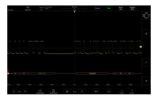
Figure 12-16 CAN bus decode interface
