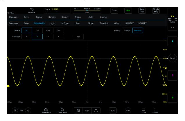
Figure 6-15 Negative Polarity Pulse Level Flip
