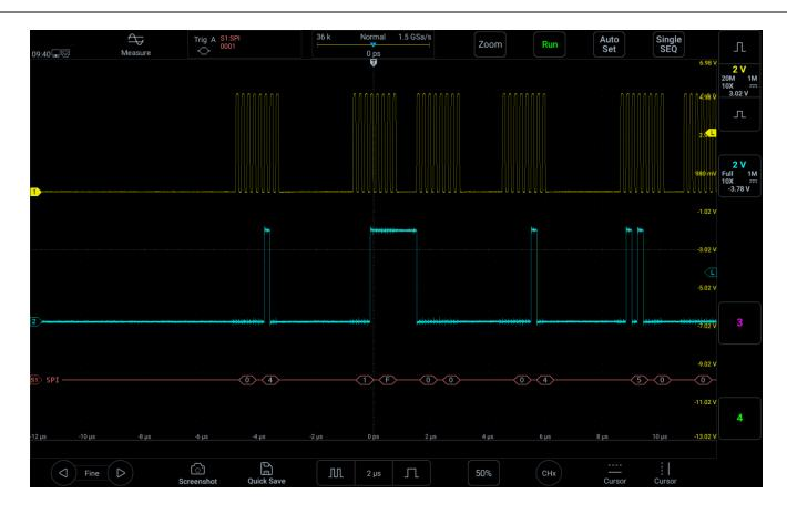
Figure 12-20 SPI bus decode interface
