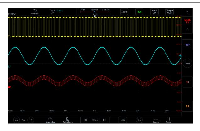
Figure 9-2 Mathematical Operation of CH1 adding CH2
