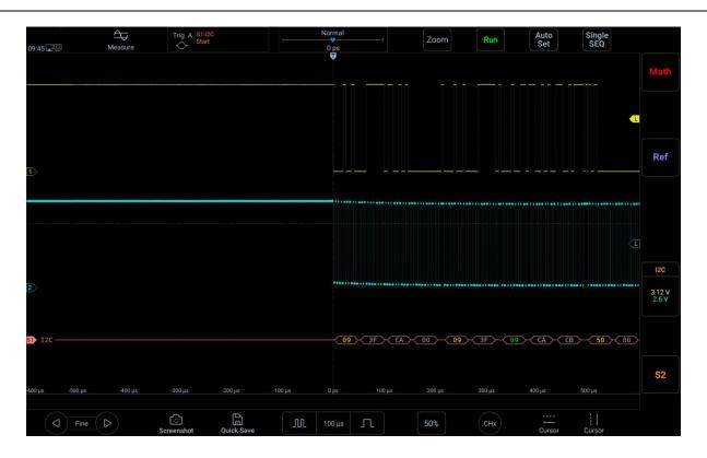
Figure 12-24 I<sup>2</sup>C Graphic Interface
