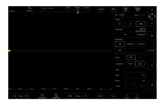
Figure 5-9 GND Coupling
