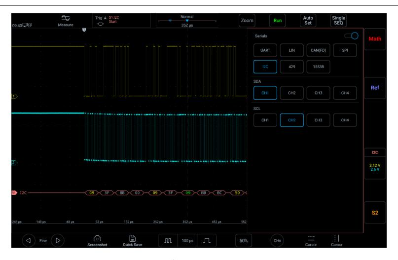
Figure 12-22 I<sup>2</sup>C Bus Configuration Menu
