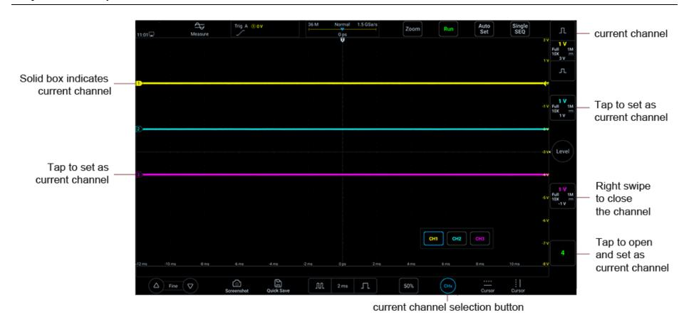
Figure 5-4 Channel Open, Close and Switching
