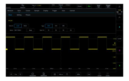
Figure 8-5 Save CH1 Reference Waveform Interface
