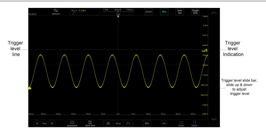
Figure 6-8 Trigger Level
