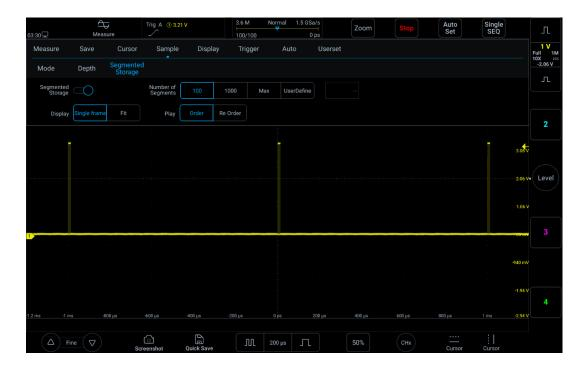
Figure 11-11 Segmented storage waveform acquisition
