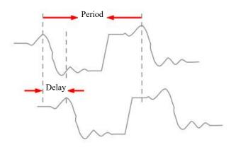
Figure 7-6 Phase Measurement Schematics
