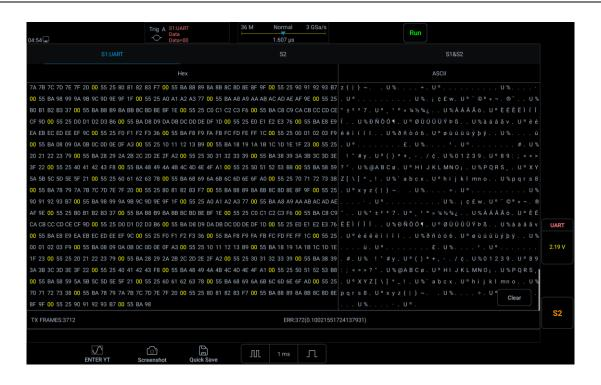
Figure 12-2 Bus Decode Text Mode
