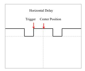
Figure 6-7 Horizontal Delay
