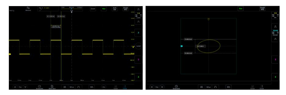
Figure 7-18 Cursor Measurement Pulse Width
