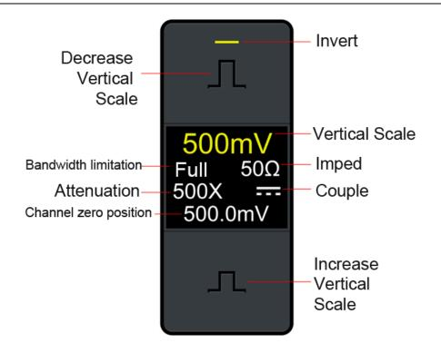
Figure 5-3 Channel Display Interface
