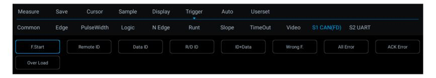
Figure 12-15 CAN FD Trigger Mode Configuration Menu
