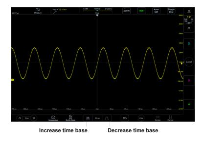
Figure 4-2 Adjust the Horizontal Time Base
