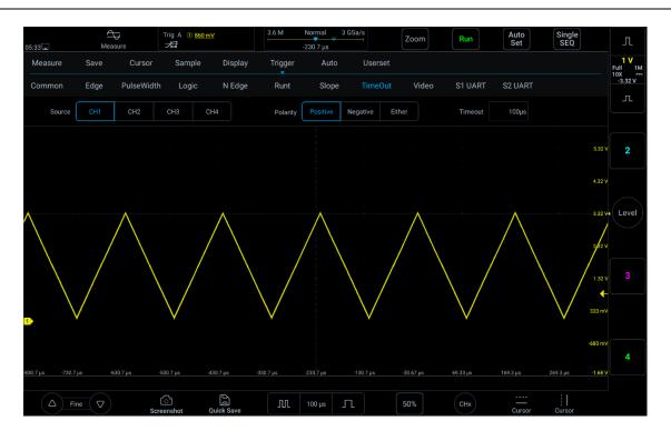
Figure 6-29 Time-out Trigger
