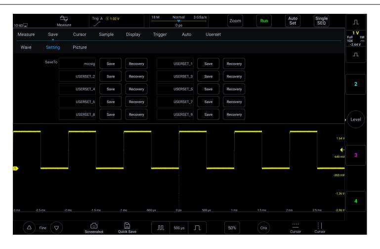
Figure 8-7 oscilloscope setting save
