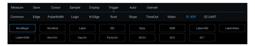
Figure 12-27 ARINC429 Trigger Mode Configuration Menu
