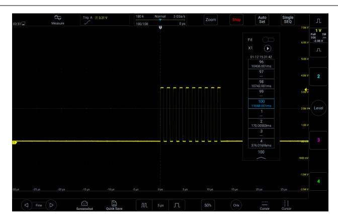
Figure 11-12 Segmented storage single frame viewing
