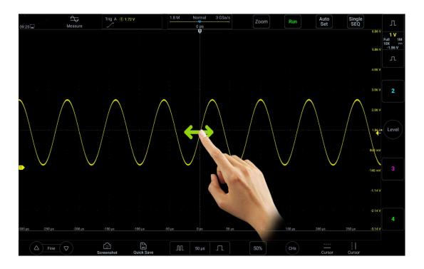
Figure 4-1 Move the Waveform Horizontally on the Screen
