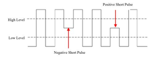
Figure 6-24 Runt Trigger
