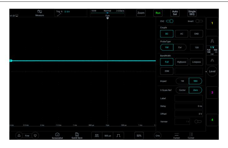
Figure 5-17 Channel input impedance
