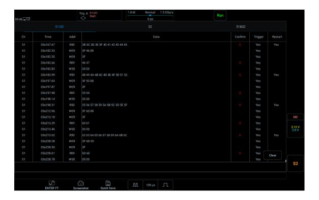
Figure 12-25 I<sup>2</sup>C Text Interface
