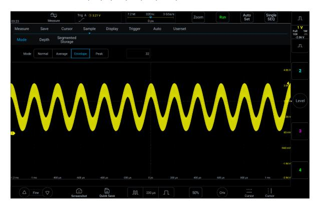
Figure 11-8 Signal in Envelope Sampling Mode (32)
