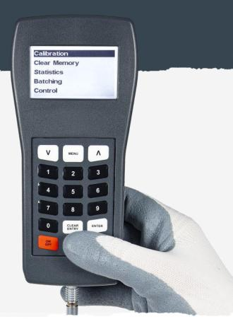
To exit from the menu, press the Menu button again and the Coating Thickness Meter will revert back to normal measurement mode.
